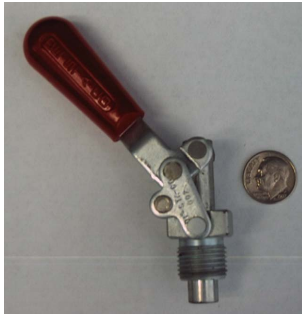
Fig. 1. The DE-STA-CO 602 straight line action clamp has an 889 N capacity.
